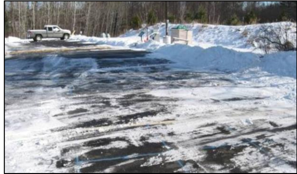
Figure 5 - Porous asphalt (left) and dense mixed asphalt (right) parking lots shown one hour after plowing on a 25° F day in February, 2007. Source: University of New Hampshire Stormwater Center
