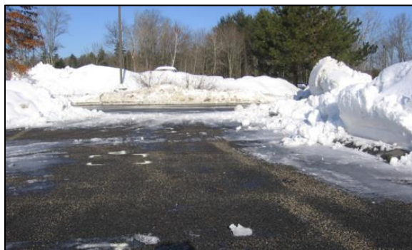
Figure 6 - Porous asphalt (left) and dense mixed asphalt (right) parking lots shown after a spring rain on snow event Source: University of New Hampshire Stormwater Center
