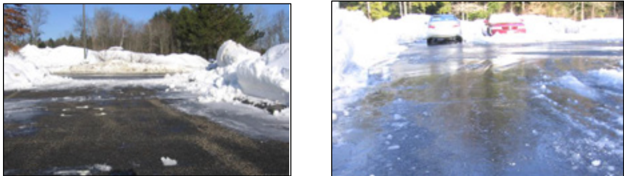
Figure D-4 - Porous asphalt (left) and dense mixed asphalt (right) parking lots shown after a spring rain on snow event Source: University of New Hampshire Stormwater Center
